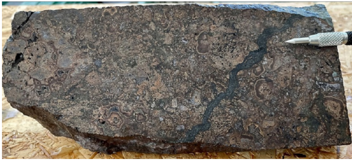
Drillhole CMVDD001. Colloform banded sphalerite with galena and stibnite.
