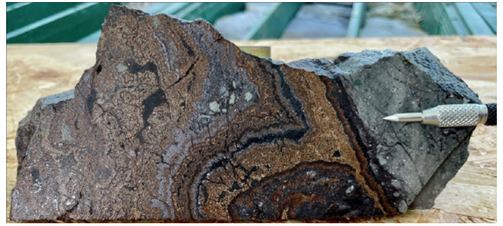
Drillhole CMVDD002. Crustiform-colloform banded sphalerite and galena.
